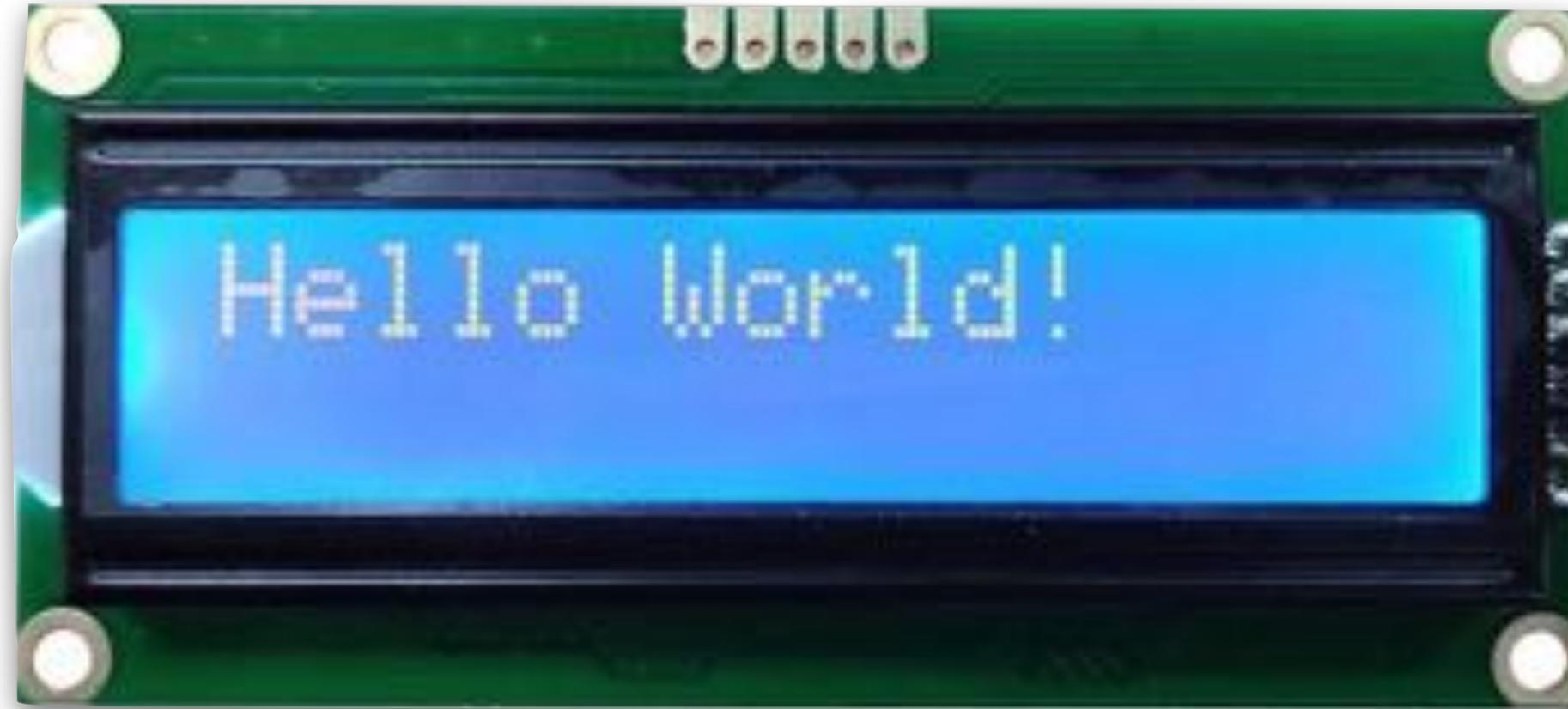
I2C and SPI 1602 Serial Character LCD for Micro:bit
