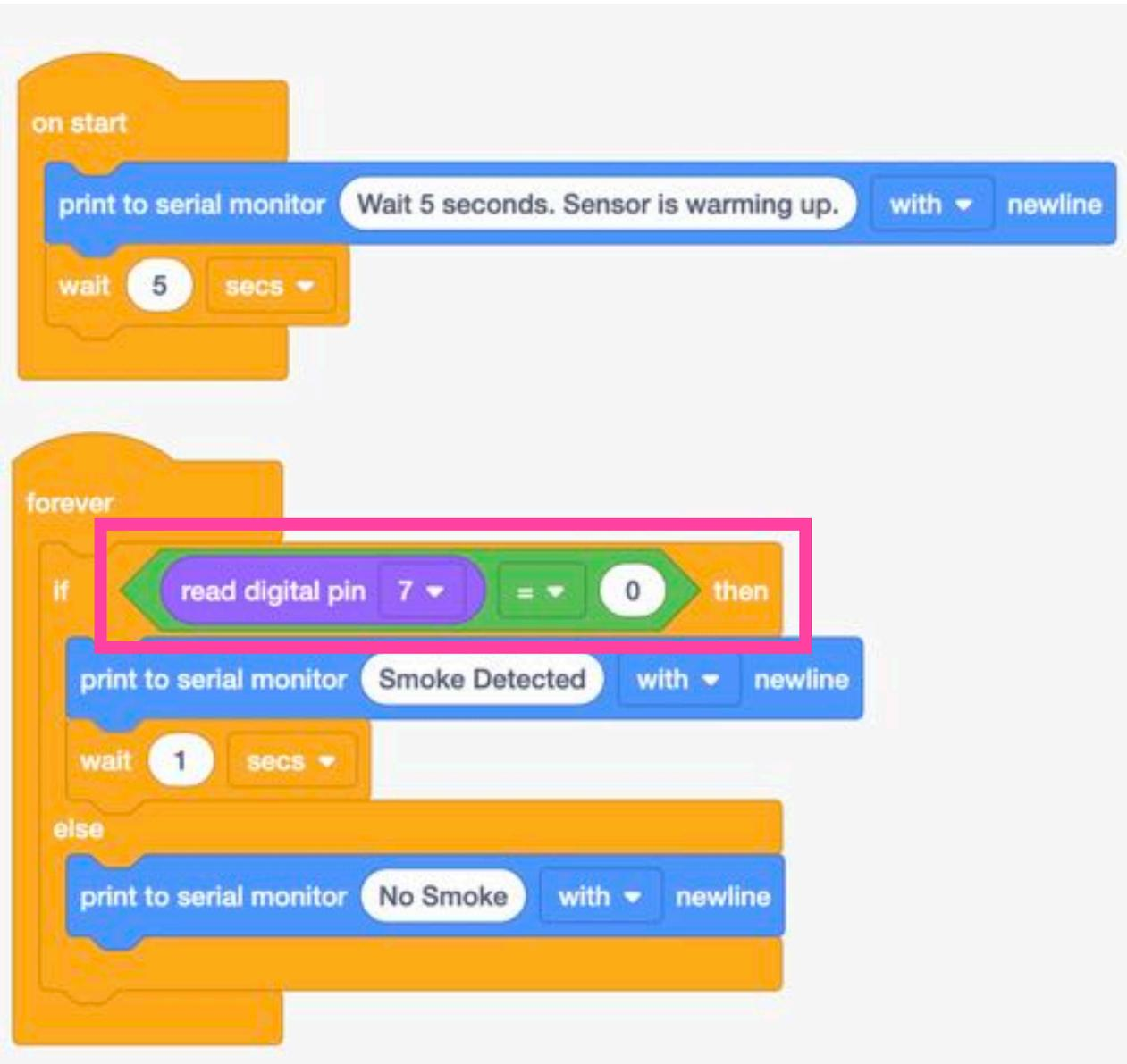
1. We are reading digital pin 7, to which the DO pin of the MQ2 sensor is connected
